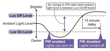
The detector measures the overall light level in the detection area and calculates the correct output for the luminaires, to achieve a preset lux level (maintained illuminance or daylight harvesting).
