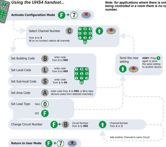
Note: for applications where there is only one channel of lighting being controlled in a room there is no need to select the channel
